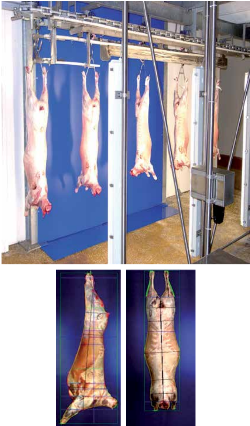
Fig. 8. Video image analysis of lamb carcasses with an E+V Technology VSS2000 system.
