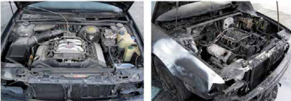
Figure 3. Engine compartment before (left) and after (right) the fire experiment
