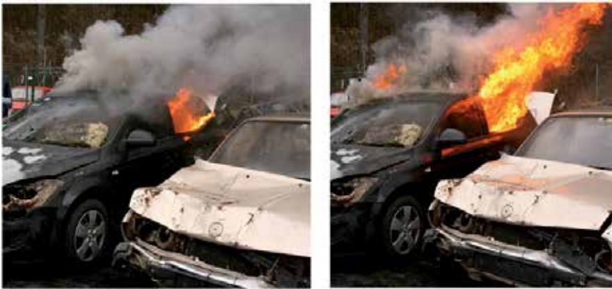
Figure 12. Full-scale fire experiment: passenger compartment fire
