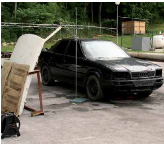
Figure 1. Automobile with thermocouples prepared for the experiment
