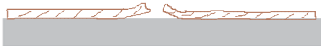
Figure 39. Schematic of debonding of composite layer at the surface near a crack
