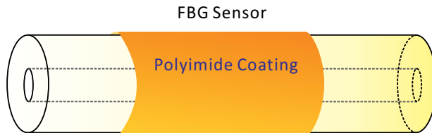
Figure 2. Illustration of a FBG sensor with polyimide coating
