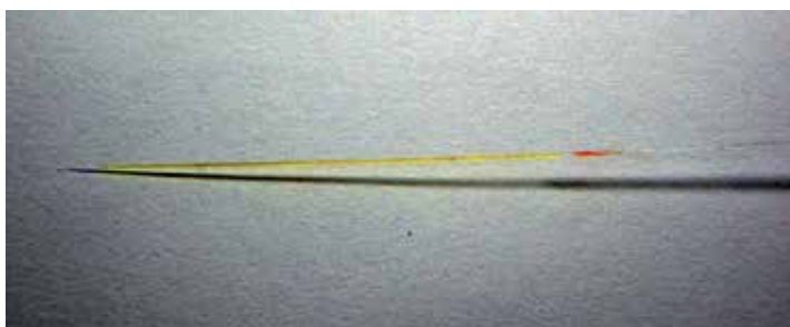
Figure 3. Photograph of fabricated FBG sensor with polyimide coating used for humidity sensing
