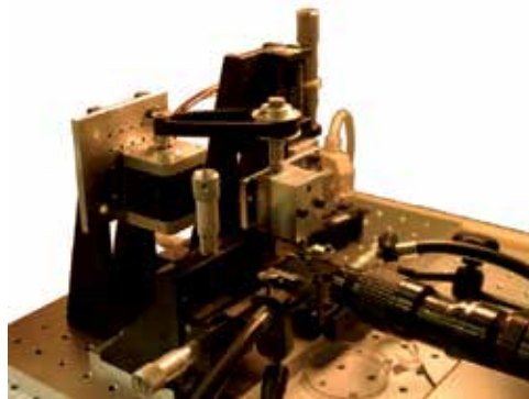
Figure 13. Experimental setup for the optical measurement of extracted trabecula in three-point bending.
