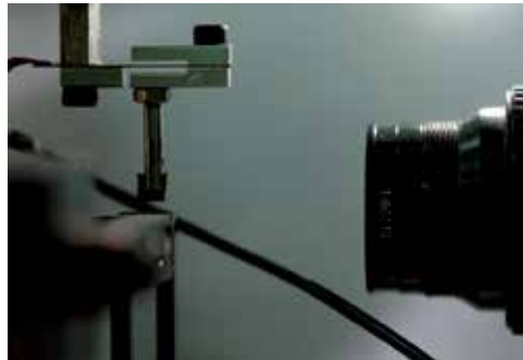
Figure 14. Close-up view of the sample showing the loading tip attached to the miniature load cell. High magnification (12 \times ) lens on right.
