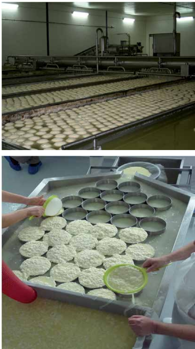
Figure 1. (Top) - Brine salting of cheeses in a large-scale plant processing 20 tons of cheese a day. (Bottom) - Small-scale unit processing 50 Kg per day of a traditional PDO cheese
