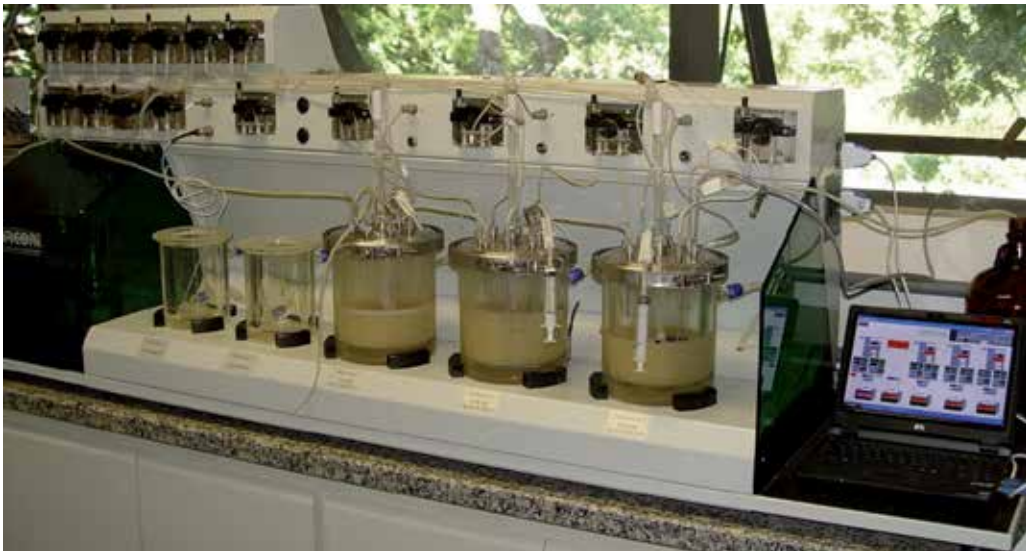
Figure 1. Computer controlled simulation of human microbial ecosystem (SHIME®) housed in the Probiotics Research Laboratory of FCF/UNESP-Brazil. Sivieri et al.[53]
