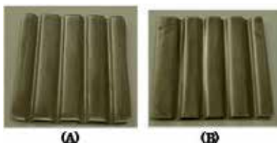
Figure 6. Photographs of the electrodes used for the initial type electrolyzer.
