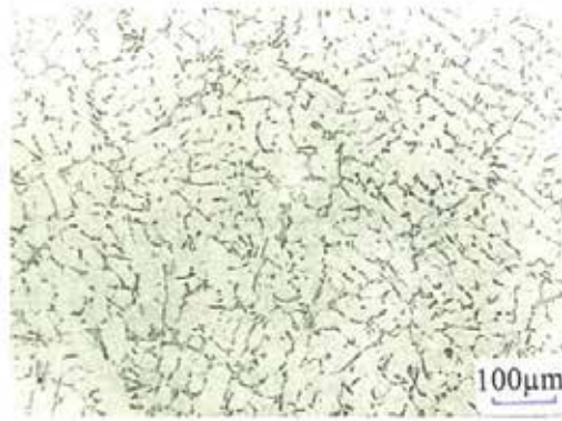
Figure 27. Optical micrograph of EA10-2 with 10% of DEASA ingot and holding time of 2hr at 720°C, indicating the unmodified structure.
