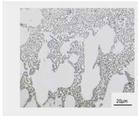
Figure 6. As-cast micrograph of EZL108 ingot, revealing self-modified structure. Optical
