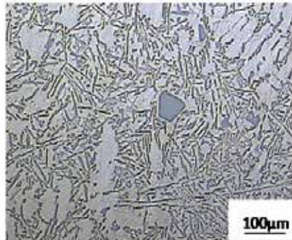
Figure 17. Optical micrograph of DEASA(EZL14) after first remelting. Self-modification is fully subjected to fading. Faceted primary silicon occurs
