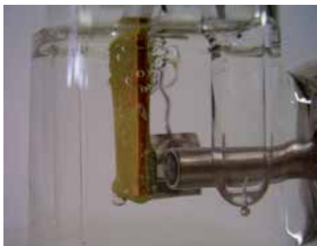
Figure 2. Ultrasound tip in front of BDD electrode (distance = 5 mm).
