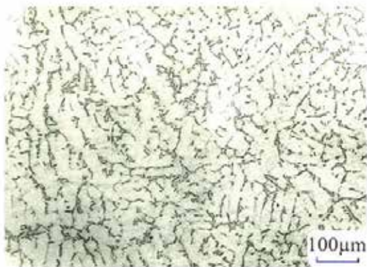
Figure 30. Micrograph of EA30-2 with 30% of DEASA ingot upon 2-fold remelting and holding time of 2 hrs, showing the modified structure. Optical.
