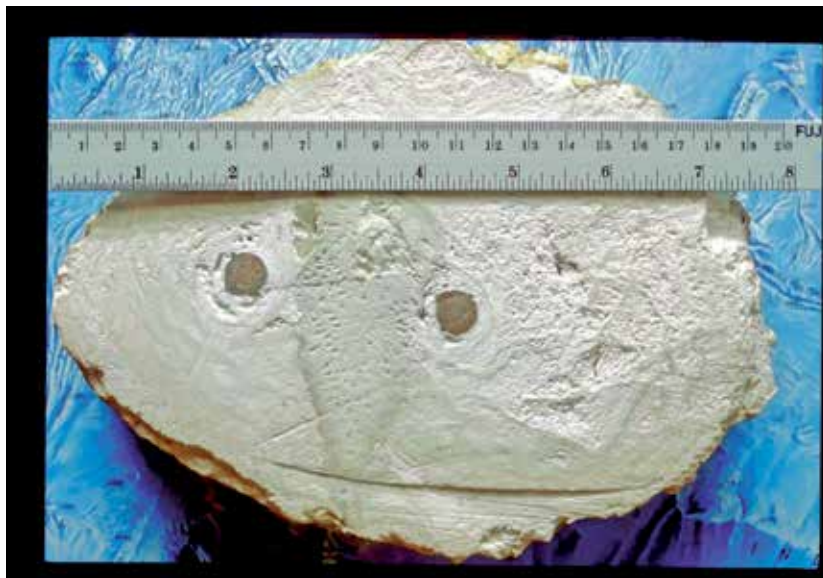
Figure 3. This piece was cut near where two steel bars crossed. We had wedged a coral between the bars after a few months of growth. The coral skeleton is the slightly darker vertically oriented area in the center. After 2.5 years it was completely overgrown and encased by electrochemically produced minerals. Photograph Wolf H. Hilbertz.
