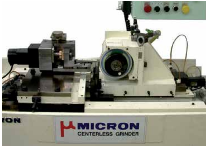
Figure 18. Photo of grinder installed a fine feed and adjustment mechanisms
