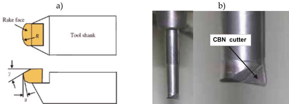
Figure 5. Tools applied in machining of carbides: a) diamond turning tool [15], b) CBN torus end mill [16]
