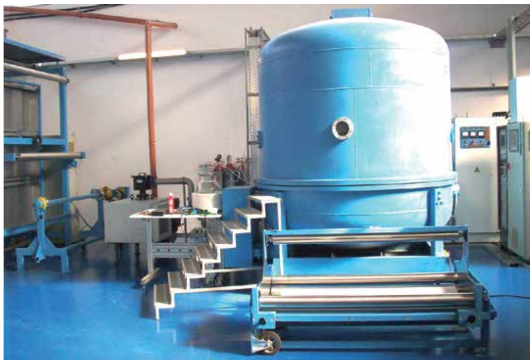
Fig. 14. Industrial plasma reactor at Textilveredelung Grabher GmbH/Austria
