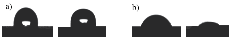
Fig. 5. Contact of water drop in the sample without (a) and with DBD plasma treatment (b) (time =0 s and after 30 s).
