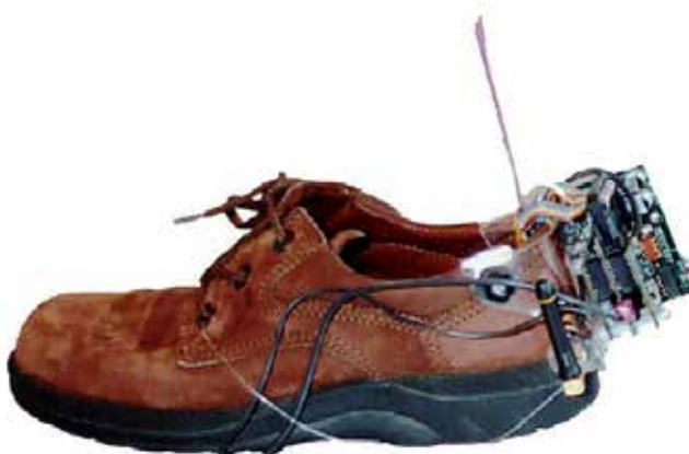
Fig. 5. Sensor Shoe, University of Twente, Enschede, The Netherlands. Gait analysis based on movement sensors (Kauw-A-Tjoe et al., 2007)
