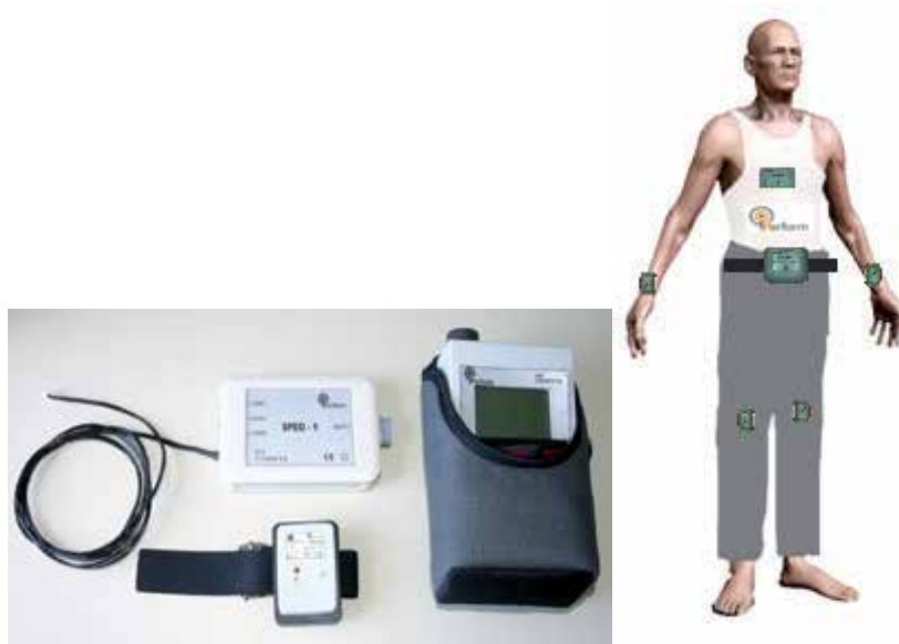
Fig. 11. PERFORM System prototype including accelerometers, gyroscope and data logger (left) System placement on the body (right)
