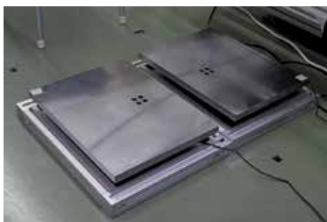
Fig. 5. Force detection plates for measuring feet pressure
