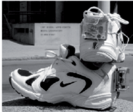
Figure 2. Piezoelectric-powered RFID shoes with mounted electronics.
