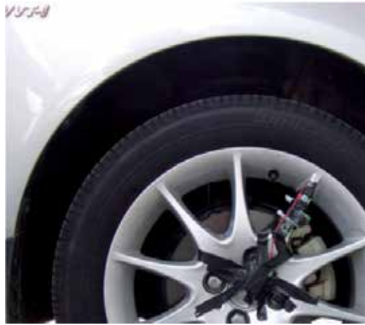
Figure 5. 3-axis accelerometer with the RF module mounted on the wheel.
