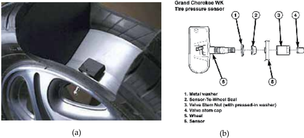
Figure 1. (a) TPMS module installed in a tire (b) Detailed components of TPMS by BMW.
