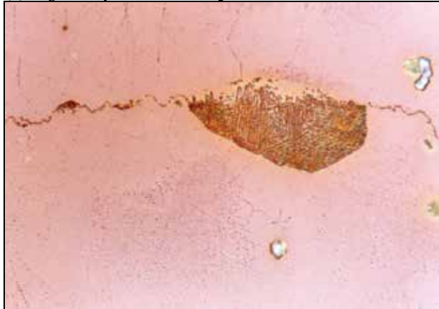
(b) Mg - alloy AZ 63HP, the plate edge, the lamellar precipitate x 500
