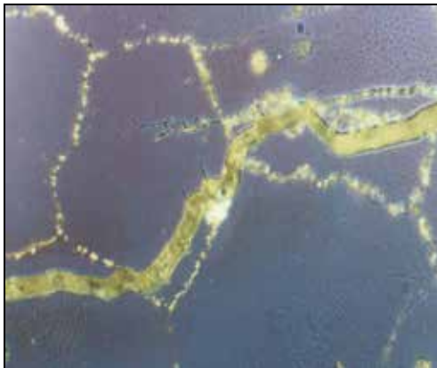
(b) transcrystalline fatigue crack growth along the grain boundaries
