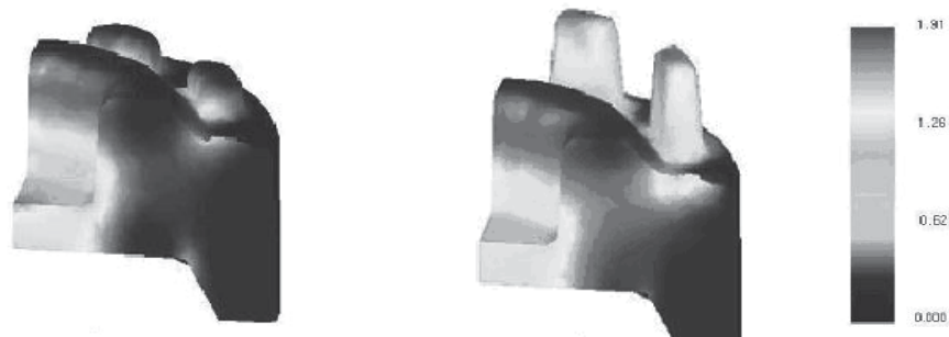
Fig. 10. Effective strain distribution of wrought magnesium alloy in traditional forging process
