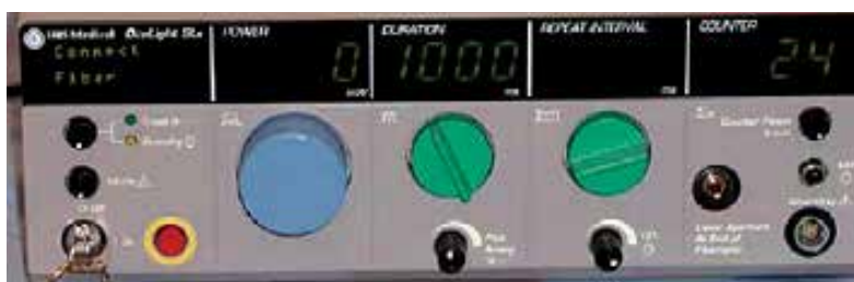
Fig. 2. Semiconductor Diode laser (IRIS Oculight SLx, Iris Medical Inc) for Diode contact TCP
