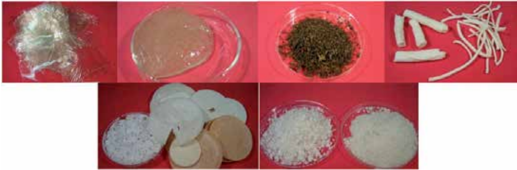
Figure 7. These are some ways you can shape the chitosan: films, gels, microspheres, tubes, sponges, powder
