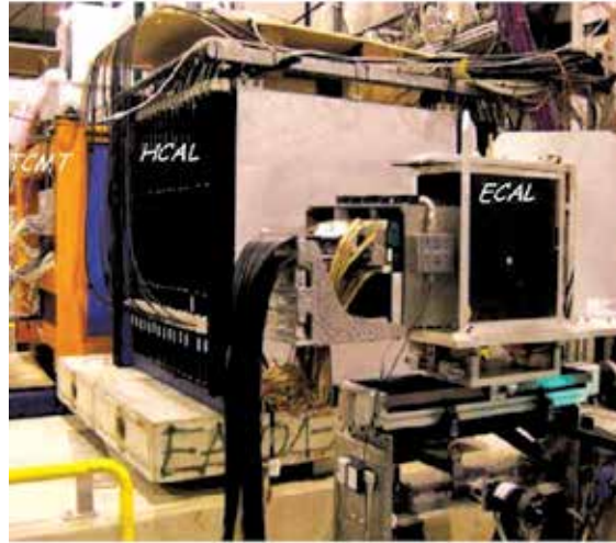
Fig. 9. Set-up of the detectors in the CERN test beam. The AHCAL was tested in combination with a prototype of highly granular Silicon/Tungsten electromagnetic calorimeter (ECAL) and a strip-scintillator/steel Muon Tracker Tail Catcher (TCMT) (Behnke, 2007).
