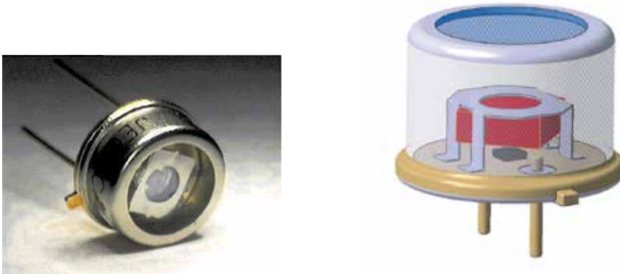
Fig. 1. (Left) Commercial hermetically sealed filtered ultraviolet (UV) photodiode with TO5 housing and the filter mounted on a metallic platform. (Right) Geometrical configuration of the photodiode. The filter crystal is here represented in red and the SiC detector dice in black. The filter is mounted on the metallic structure but does not reach the side of the housing.
