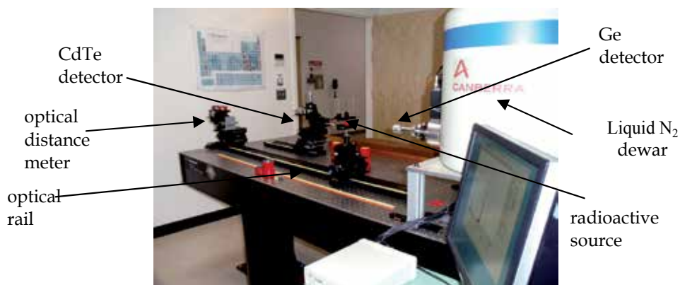
Fig. 13. Experimental arrangement for calibrating detectors using radionuclides
