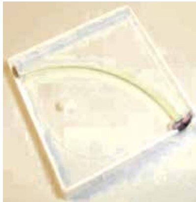
Fig. 6. Design of the scintillator/SiPM detection system for hadron calorimetry. The green sensitive SiPM is coupled to the scintillator through a wavelength shifter fiber (CALICE, 2010).
