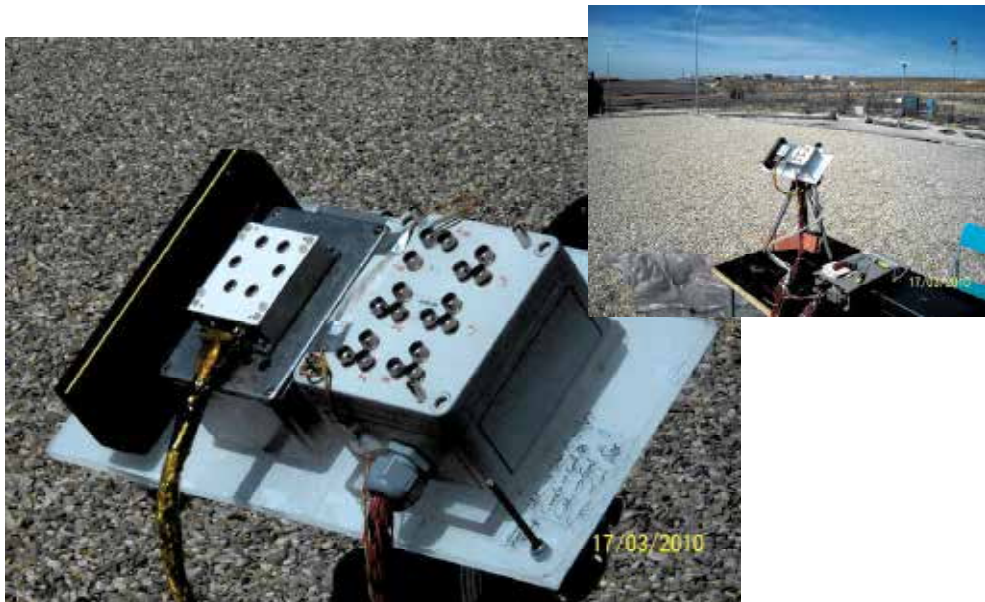
Fig. 9. Engineering model for field campaign measurements. The direct beam (Sun) angle of incidence can be varied by adjusting the platform inclination.
