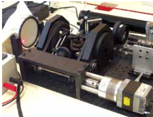
Fig. 18. Photograph of the mechanical device of the rotating texturometer used in the extensometry application.
