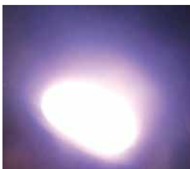
Fig. 8. Photograph of the typical glow from ZnO target when sputtering.
