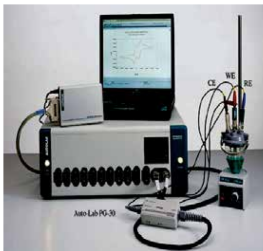
Fig. 1. Electrochemical etching setup for fabricating PS layers
