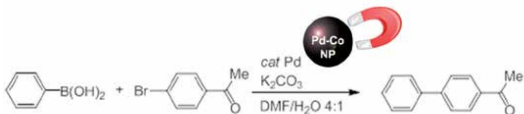
Figure 23. Suzuki reaction by using Pd or Pd@Co nanocomposites with optimized conditions.
