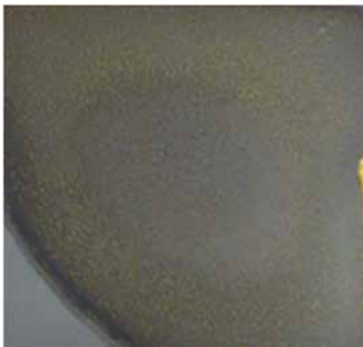
Fig. 19. The impact of pure \text{SF}_6 etch on a silver layer showing yellow (sulphur) dots in the surface
