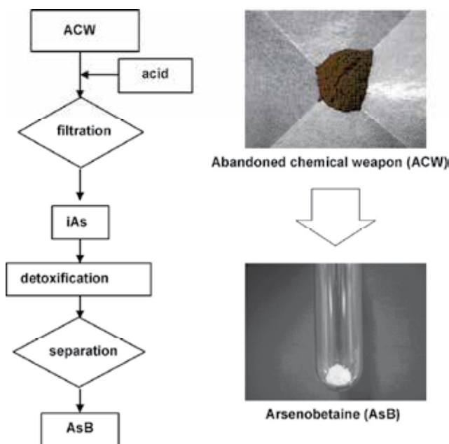
Fig. 11. Process for the detoxification of abandoned chemical weapons, the pulverized abandoned chemical weapons actually used, and the synthesized and isolated arsenobetaine.
