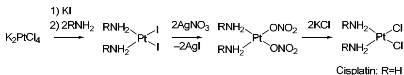
Figure 2. Synthesis of Pt(II) cis -diamino complexes.
