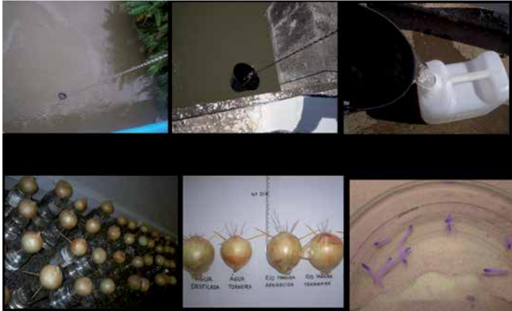
Figure 3. Allium cepa bioassay: a 20 L bucket was used for collecting the samples and transferred to 40 L containers (up); bulbs were exposed to treatment for 24 hours; growth root and root stained with Schiff (down).
