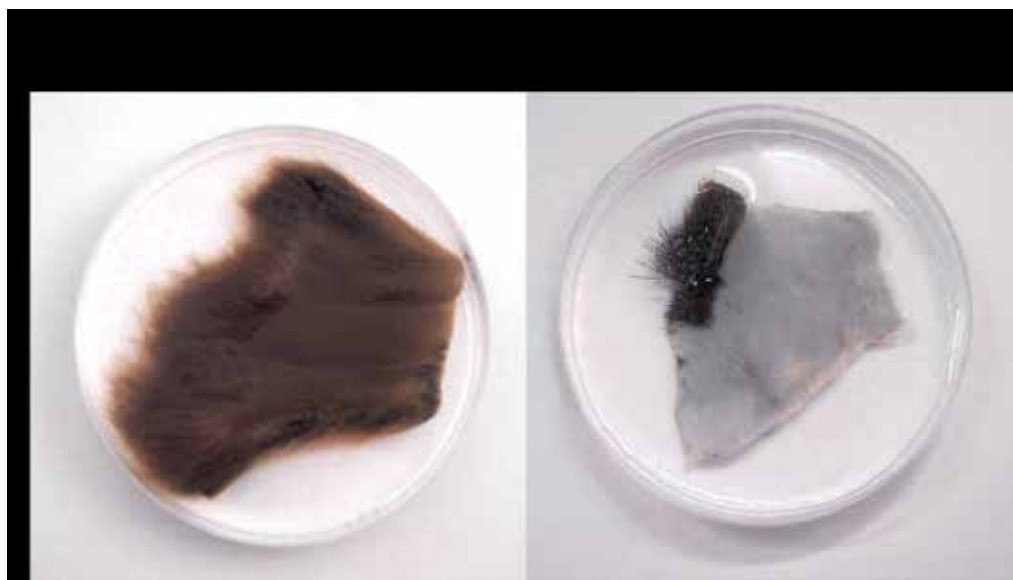
Fig. 5. Dehairing function of SAPB. SAPB was incubated for 24 h at 37°C with, goat hair. (Left = control, Right = test).
