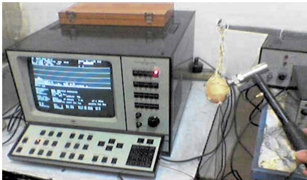
Fig. 3. (b) Free suspension for modal analysis.
