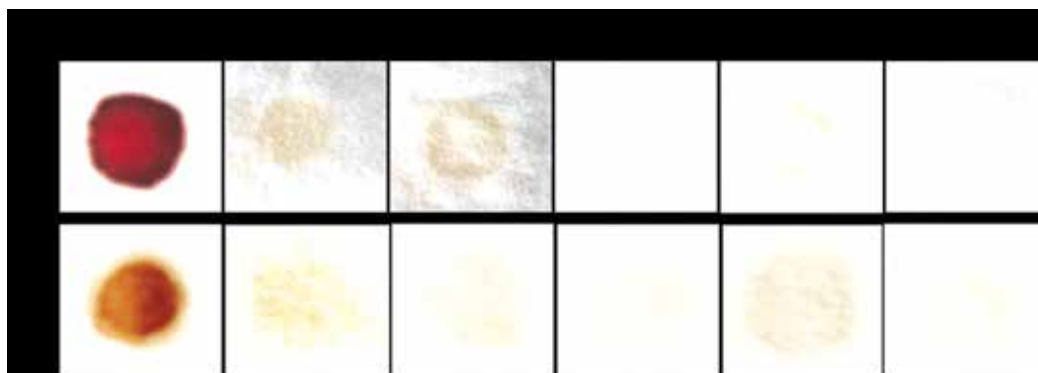
Fig. 3. Example of washing performance analysis test of SAPB. Stained cloth pieces with blood (I) or chocolate (II). (A) Control: untreated stained cloth pieces; or stained cloth pieces washed with: (B) distilled water, (C) Det detergent (7 mg/ml), (D) SAPB (500 U/ml), (E) SB 309 (commercial enzyme, 500 U/ml), and (F) SAPB (500 U/ml) + Det detergent (7 mg/ml).
