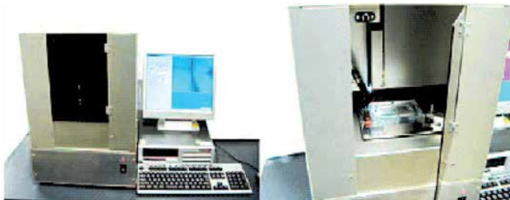
Fig. 2. Fully automated injection system for zebrafish
