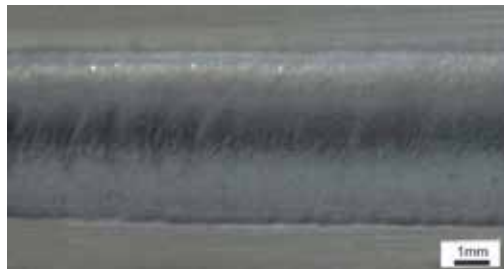
Figure 2. View of the MCMgAl12Zn1 casting magnesium alloy face of weld after laser treatment with WC, scan rate: 0.75 m/min, laser power: 1.2 kW
