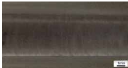
Figure 1. View of the MCMgAl9Zn1 casting magnesium alloy face of weld after laser treatment with TiC, scan rate: 0.75 m/min, laser power: 1.2 kW
