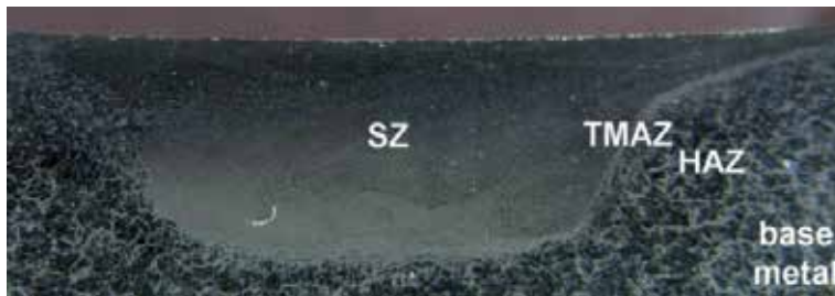
Figure 27. Various microstructural zones in the cross section of friction stir welded AZ91 alloy.
