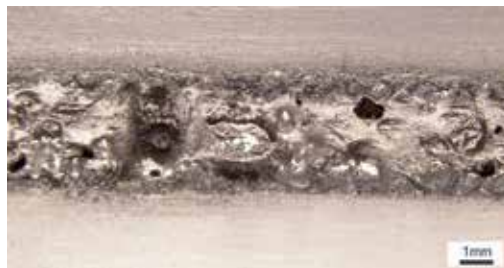
Figure 3. View of the MCMgAl9Zn1 casting magnesium alloy face of weld after laser treatment with WC, scan rate: 1.0 m/min, laser power: 2.0 kW
