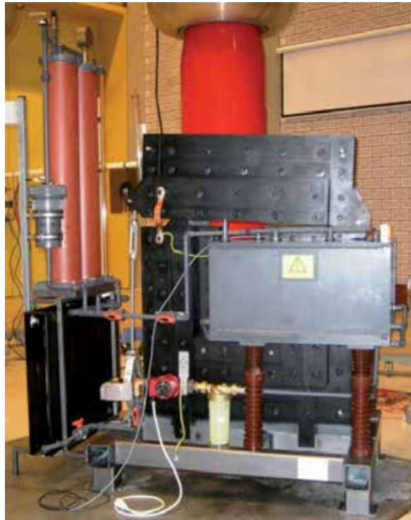
Figure 9. The resonant coil - a key ICAAS component
