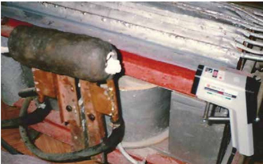
Figure 13. The inductor during the heating process
