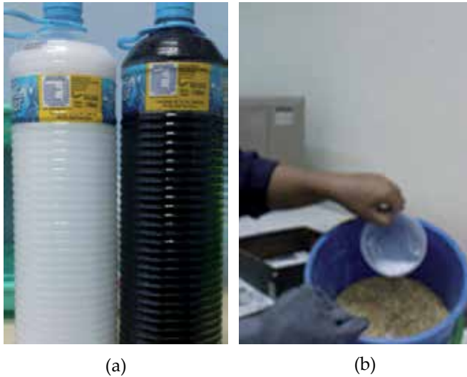
Figure 6. (a) Urea Formaldehyde and Phenol Formaldehyde resins (b) resin -paddy waste mixture
