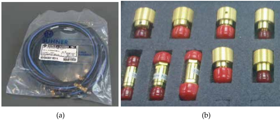
Figure 10. (a) coaxial cables (b) Agilent 85052 D calibration kit
