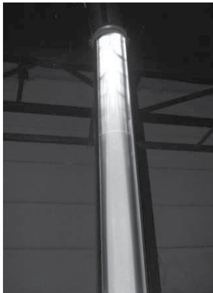
Figure 7. Prismatic light tubes are used for transporting and distributing natural light. Experimental setup in the School of Optics (Complutense University of Madrid)
