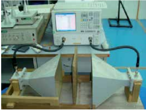
Figure 12. Free Space Measurement Setup
