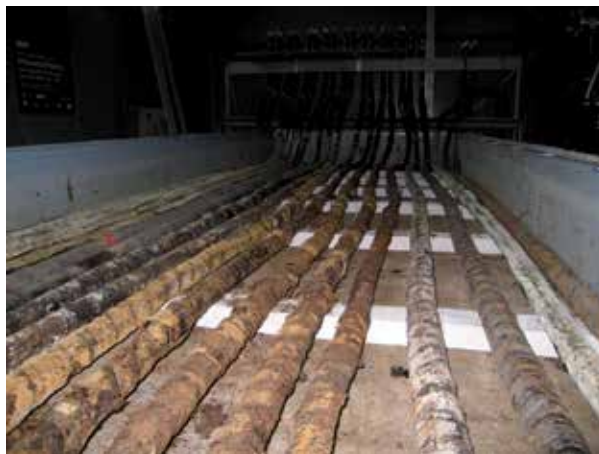
Figure 10. Cable samples in the thermal tank of the ICCAS system
