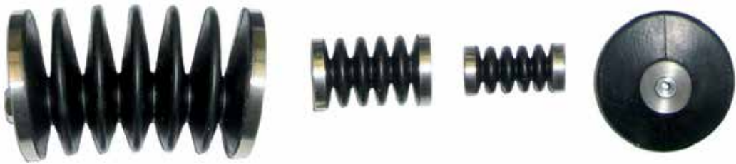
Figure 17. Series of Vulcanized FFAs: (from left to right) 36mm, 18mm, 11mm, and single chamber FFA
