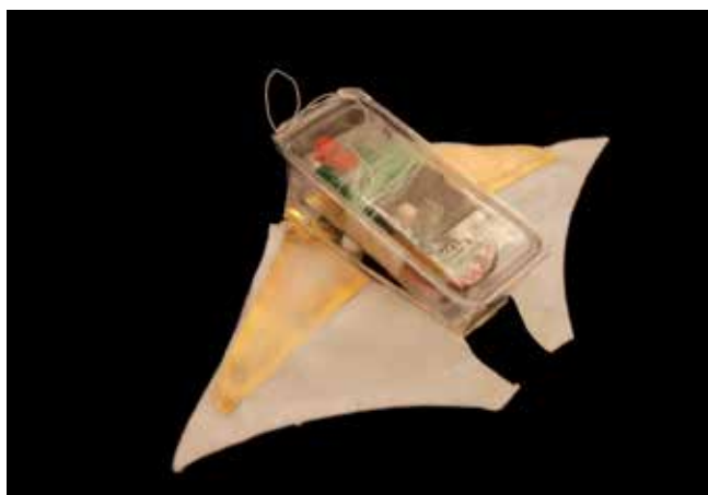
Figure 15. Free swimming robotic manta ray body.
