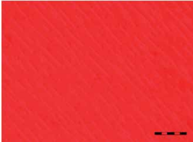
Figure 3. Microscopic picture upon magnetic field application of an inverse FF consisting of PMMA microparticles dispersed in a FF (5 vol % of magnetite in mineral oil). It can be seen that the non-magnetic particles (white spots) form chains in the direction of the magnetic field. Bar length: 100 \mu\text{m} .
