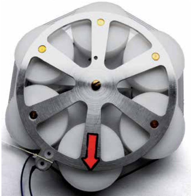
Figure 8. Amagnetic SMA rotary actuator, consisting of two coils of wire traversed by the same current in opposite directions. This arrangement produces self-annihilation of induced magnetic fields.
