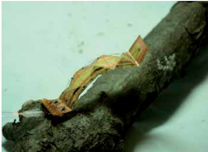
Figure 8. Omegabot, a biomimetic inchworm robot, grasps the branch of a wood, raises its head, and turns right. Bottom right: Proleg of Omegabot [38].
