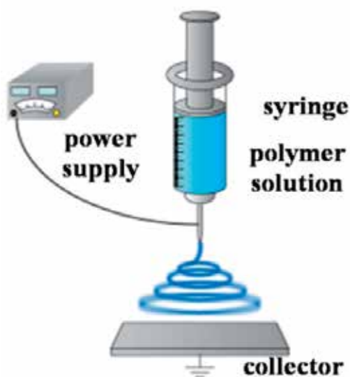
Figure 5. Schematic illustration of electrospinning set-up.
