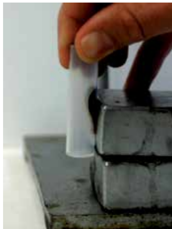
Figure 2. FF (5 vol % of magnetite) subjected to magnetic field application by a powerful rare-earth magnet. It can be seen that the liquid moves as a whole towards the zone where the field is more intense.
