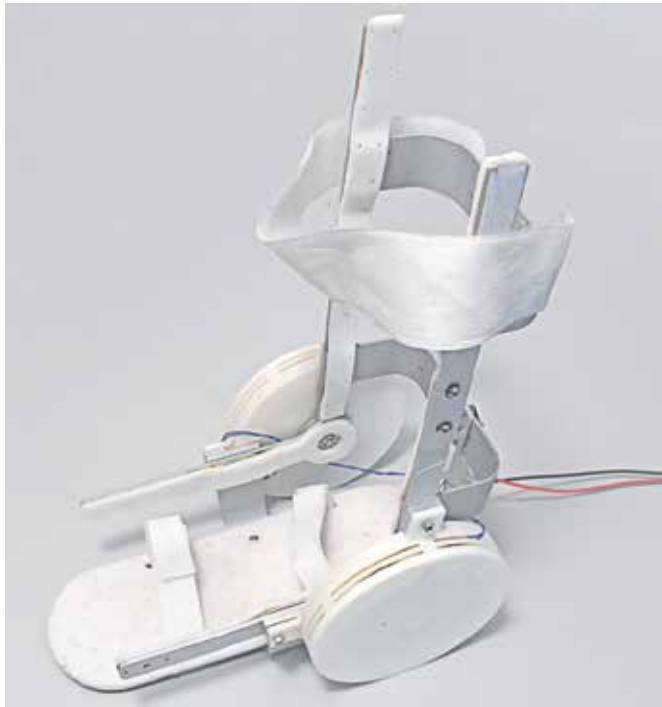
Figure 7. Implementation of an amagnetic device for ankle dorsiflexion with rotary actuators
