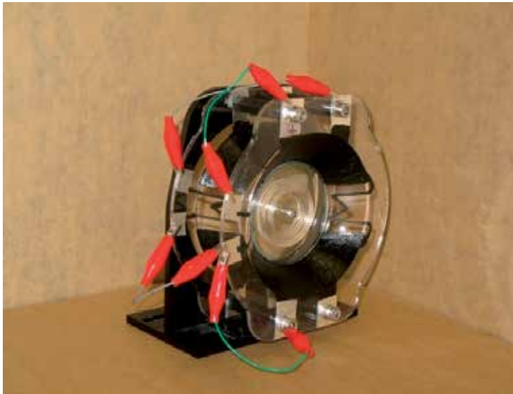
Figure 7. A photograph of a soft generator prototype. The large black regions are the generator electrodes and the thin "M-shaped" electrodes are the piezo-resistive switches.
