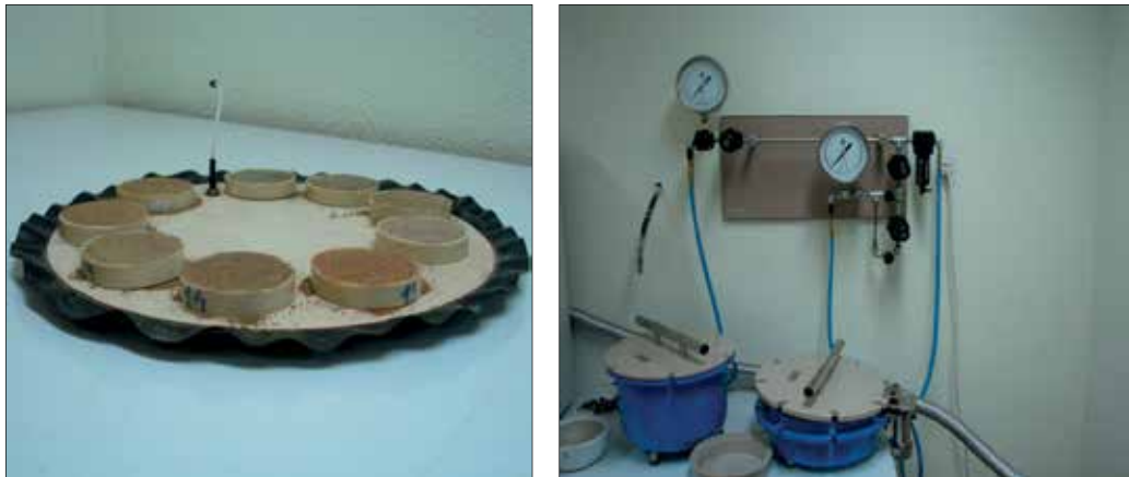
Figure 2. Preparing soil and placing samples on Bar extractor and Porous plate extractor
