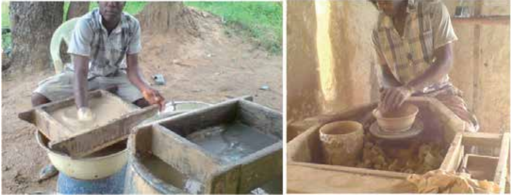
Figure 13. Local clay body preparation and clay throwing process at Maraba Pottery Centre
