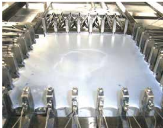
Figure 17. The table tenter used for biaxially-stretching the sheets.
