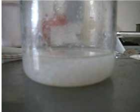
Figure 15. Swelling of the CNF compounded HDPE pellets with liquid paraffin.
