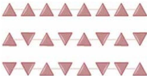
Figure 2. Representation of an isotactic polymer (top) where all monomers have the same stereo/regiochemical configuration, a syndiotactic polymer (middle), where the monomers have alternating positions along the chain and an atactic polymer (bottom) where the configuration of the monomers is random.
