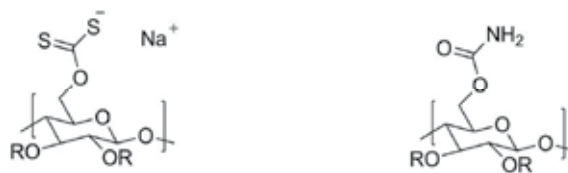
Figure 1. Cellulose xanthogenate (left) with R = H or xanthogenate group and cellulose carbamate (right) with R = H or carbamate group.
