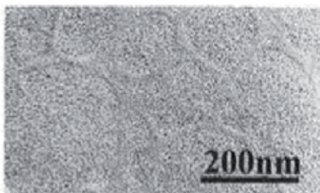
Figure 5. TEM image of the palmitoyl cellulose LB films deposited at 293K. Circle areas are palmitoyl cellulose grains.
