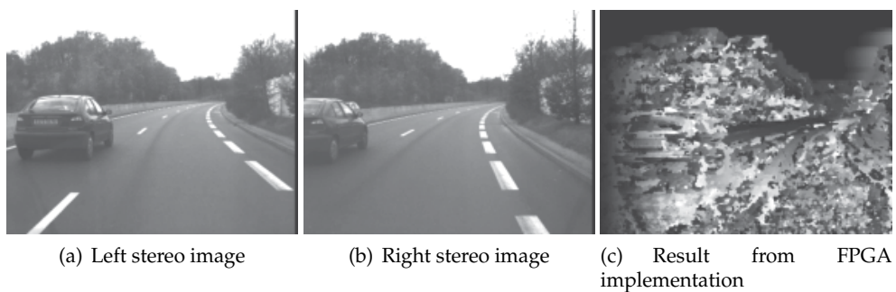
Fig. 10. Stereo images acquired from a vehicle in the highway: a) left image b) right image and c) the disparity map.
