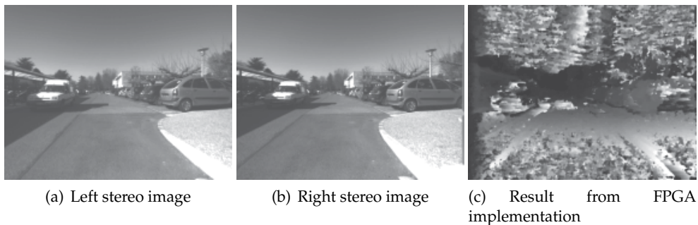
Fig. 9. Stereo images acquired from a mobile robot during outdoor navigation: a) left image b) right image and c) the disparity map.
