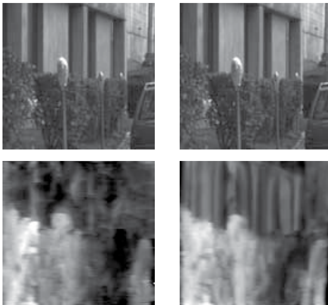
Fig. 6. Top: Meter stereo pair. Bottom: Disparity maps obtained through the whitened Green's function approach (left) and through the original approach of (Torreão, 2007) (right).
