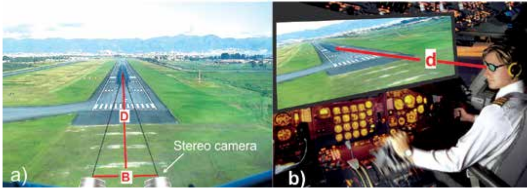
Fig. 6. Idealized flight simulator during a landing maneuver. a) Registering images in a stereo camera. b) Viewing stereo images in a three-dimensional screen. Variables B , D and d , influencing E' , are indicated in red.
