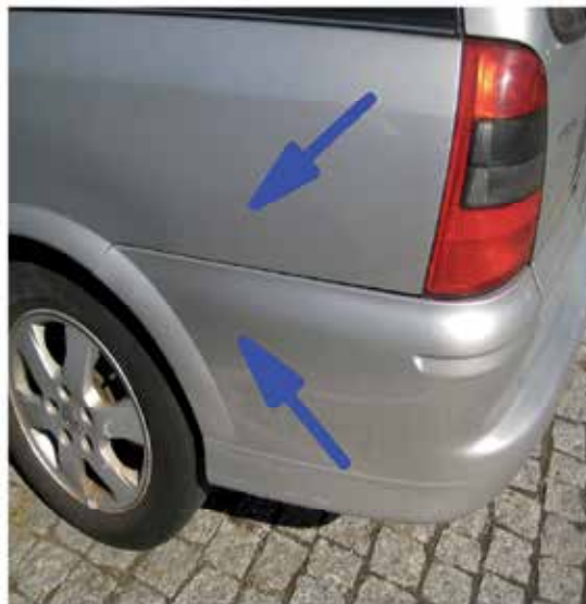
Fig. 3. Example of colour harmony in a silver-like coating containing aluminium flakes. Current colour designs must achieve no perceptible colour differences between the different external parts that integrate the car such as the car body and the fenders.
