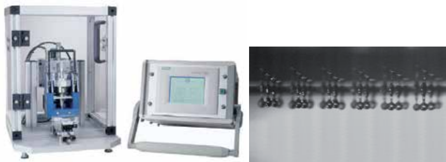
Fig. 2. The Topspot/E (left) and the formation of droplets from the print head (right).
