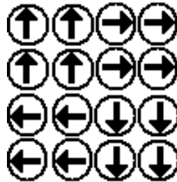
Fig. 14. Ordering of the atomic dipoles in a superparamagnetic material.
