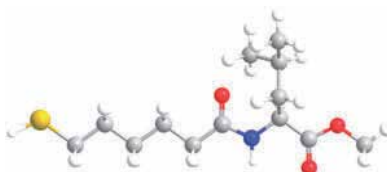
Fig. 8. S-leucine methyl ester covalently attached to 6-mercaptohexanoic acid (S-LMHA). Red atoms = oxygen, blue =nitrogen, gray = carbon, yellow = sulfur, white = hydrogen. (Ejgenberg and Mastai, 2011)
