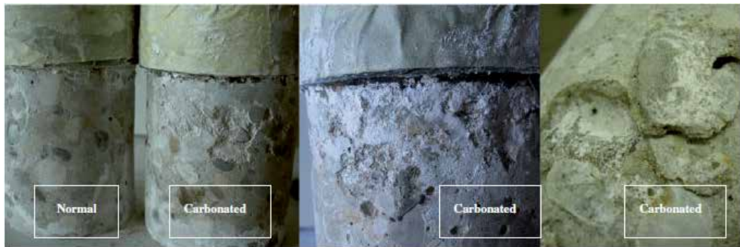
Fig. 17. Visual observation of normal and carbonated concrete specimens exposed to sodium sulfate solution [53]
