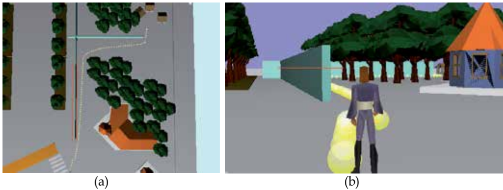
Fig. 13. An example path generated by the path planner: (a) avoiding the obstacles described by the 2D approximation in semantics; (b) a snapshot of the scene from the avatar's view.
