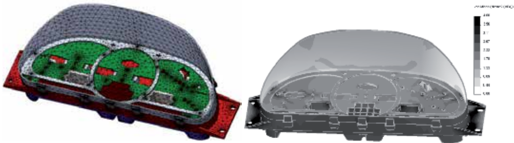
Fig. 15. Meshed 3D model and von Mises stresses distribution in initial design of GP.
