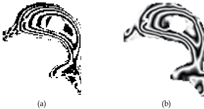
Fig. 15. (a) Result of binarize fig 14; (b) Fringe pattern associated with the demodulated phase.
