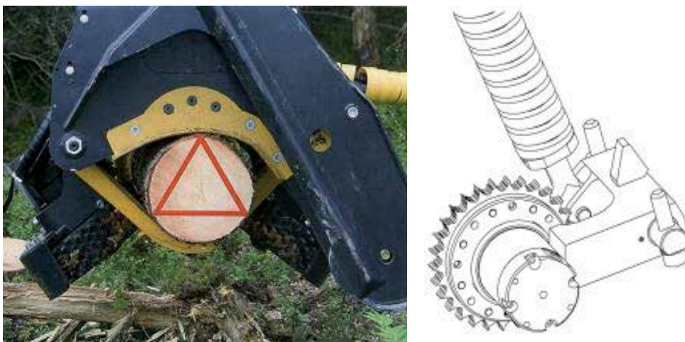
Fig. 2. Photo + scheme of scanning the stem diameter and length at harvesters (both figures according to Ponsse).
