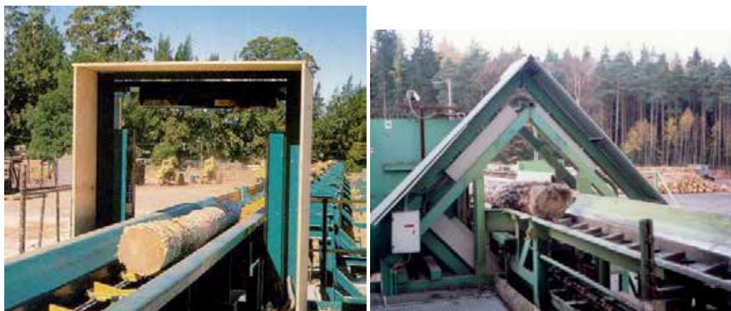
(a) vertical and horizontal position of scanning systems (b) placing the scanning systems at an angle of 45°
