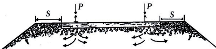
Fig. 6. Changing the location of ballast under the load of passing train
