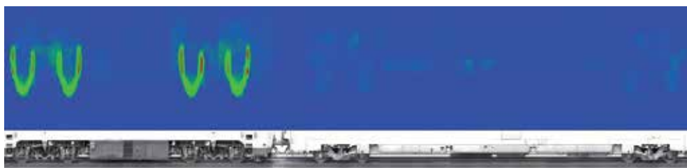
Fig. 4. Example of thermal acquisition of the lower part of a train (thermal map, upper, and visual image, lower).
