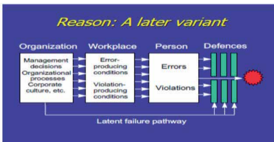
Fig. 2. A reference Model for Accident Analysis. Sourced from (Wikipedia 2011).
