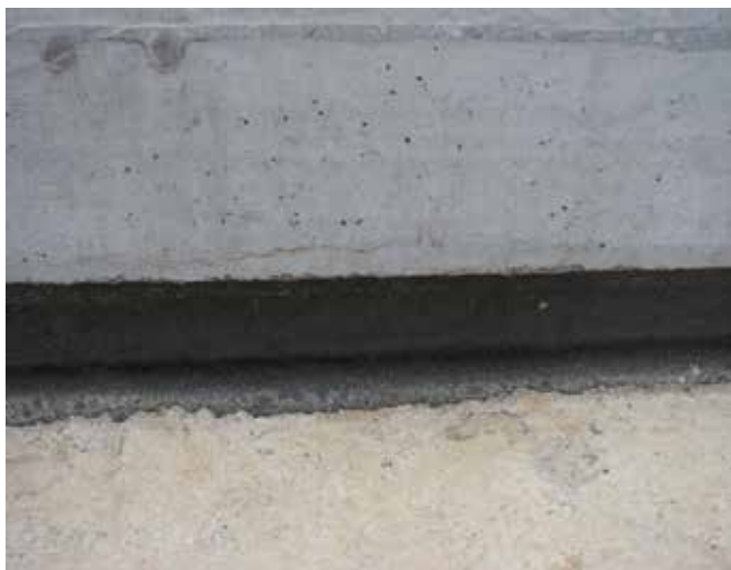
Fig. 39. Harden state of CA mortar
