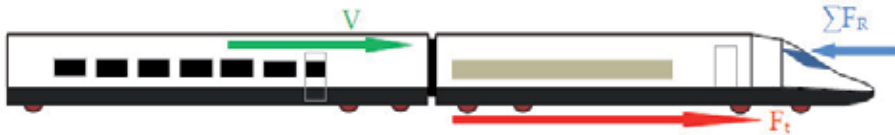
Fig. 1. Longitudinal train dynamics.
