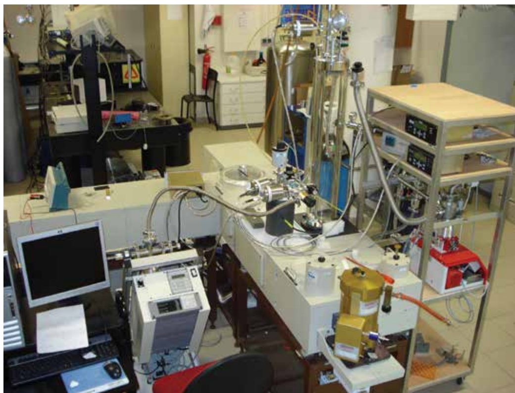
Fig. 3. View of the laboratory showing the Fourier transform spectrometer Bruker IFS125HR, two multiple-reflections Pyrex absorption cells and a gas handling system including a turbomolecular pump. In the back is an optical table with a difference frequency generation (DFG) laser system developed at LPPM in Orsay and LISA in Créteil
