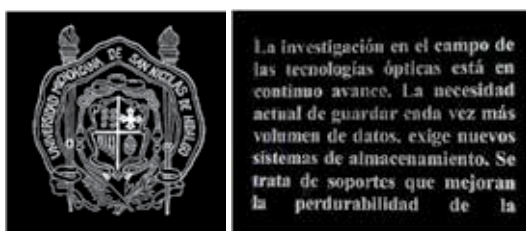
Fig. 23. Binary objects employed to Fourier holograms recording.
