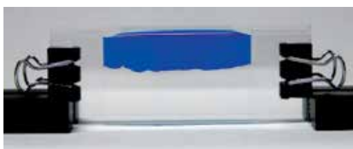
Fig. 5. Photography of the emulsion between two glasses deposited by gravity technique.
