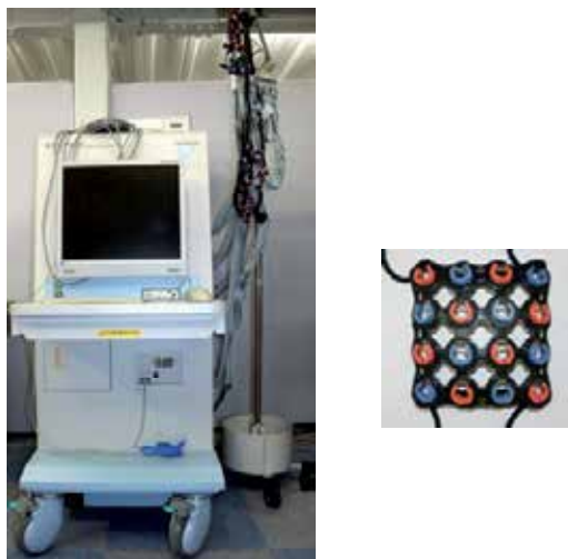
Fig. 4. ETG-7100 system and its shell to hold 4×4 optodes.
