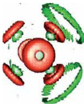
Fig. 9. Structure of [Ni(H 2 O) 6 ] 2+ complex showing also the second hydration shell around the complex. Green – oxygen in water, Red – hydrogen in water For details see the text.
