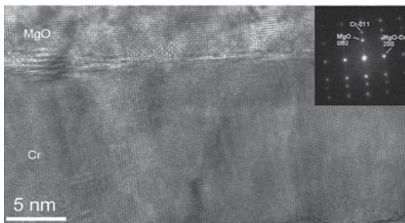
Fig. 6. High Resolution Transmission Electron Microscopy image of an MgO//Cr film deposited at room temperature and annealed at 600°C, confirming the single crystalline growth of Cr on MgO (by courtesy of E. Snoeck CEMES, TOULOUSE).
