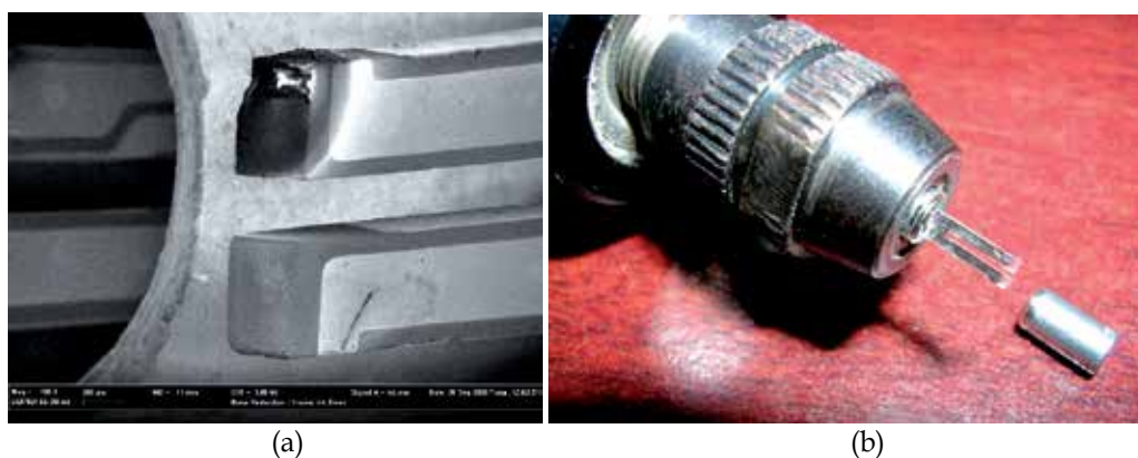
Fig. 2. (a) SEM image of tuning fork displaying the layout of the electrodes. (b) A tuning fork just removed from its packing, and the metallic enclosure that would otherwise keep it under vacuum.
