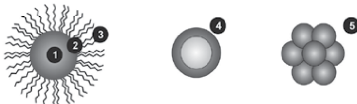
Fig. 1. Reactivity of Colloidal Inorganic Nanoparticles. The critical factors to consider on the study of INP's reactivity are i) Effects of inorganic core's size and shape, ii) the surface molecule substitution and ligand exchange, iii) the particular reactivity of the coating molecule, iv) the interactions with ions present in the colloidal solution and v) cooperative effects with other NPs present in solution.
