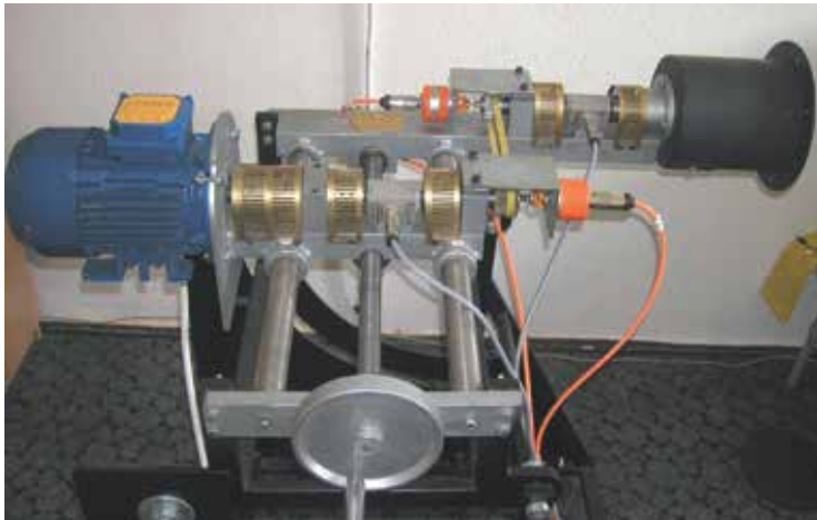
Fig. 15. The station of the general-purpose laboratory grinder ULR-2,0/2004 - with horizontal position of the drive shaft
