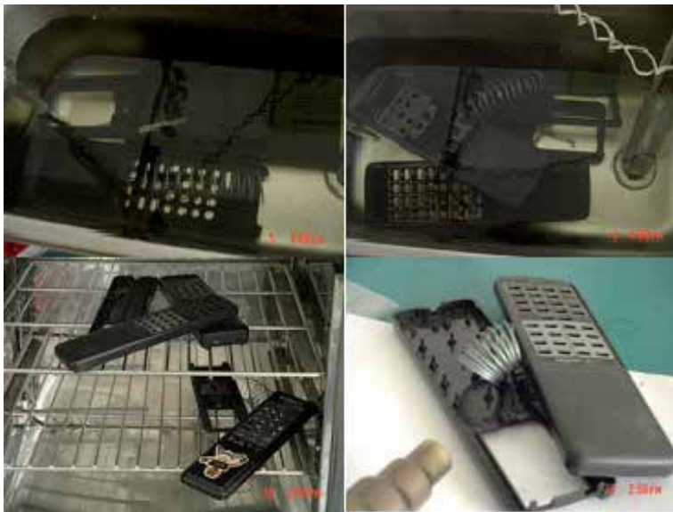
Fig. 1. The active disassembly efficiency of the shells of remote controls (G. Liu et al., 2008).
