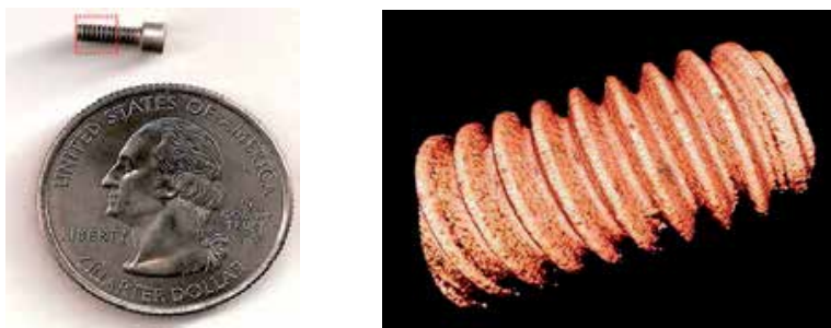
Fig. 3. 3D optical profiling of an M2 metal screw. Photos used with permission of Thorlabs®.
