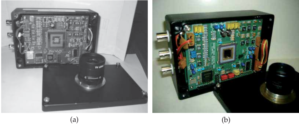
Fig. 2. Photographs of CIS cameras with CMOS chips of (a) 64 \times 64 -pixel and (b) 200 \times 200 -pixel sensors.
