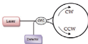
Fig. 3. A schematic diagram of Sagnac fiber interferometer.
