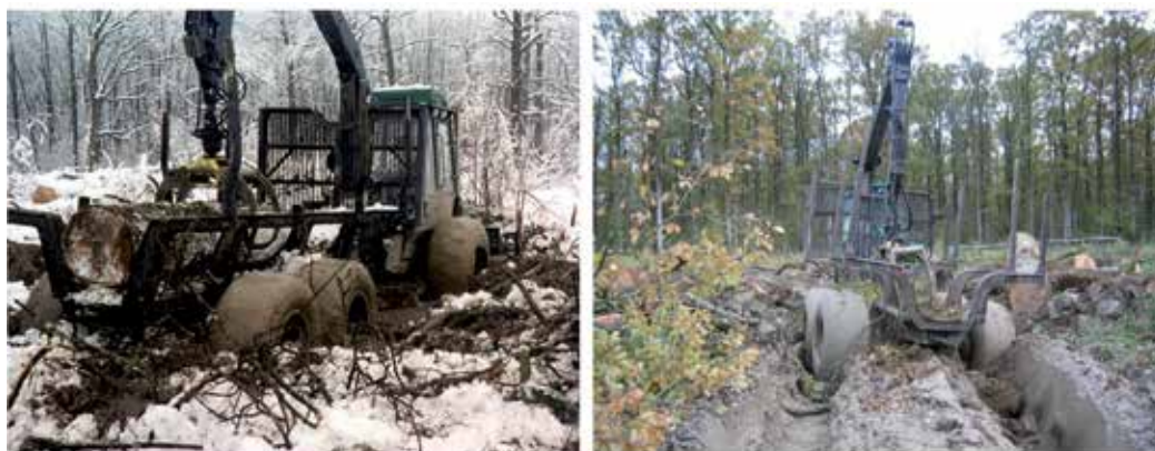
Fig. 1. Forwarder mobility and soil disturbance in main felling of lowland even-aged forests of Croatia
