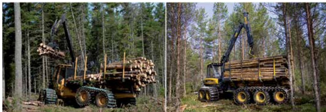
Fig. 8. Eight and ten wheeled forwarder with semi-tracks
