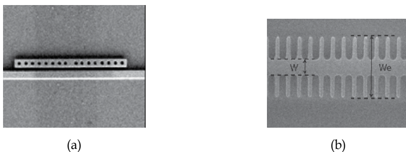
Fig. 2. SEM pictures of two planar 1D periodic structures used for sensing purposes. (a) 1D SOI holes cavity (Goddard et al., 2010); (b) 1D SOI corrugated waveguide (Castelló et al., 2011).
