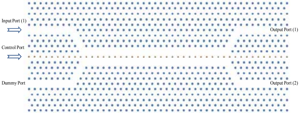
Fig. 7. The all-optical switch designed using a directional coupler.
