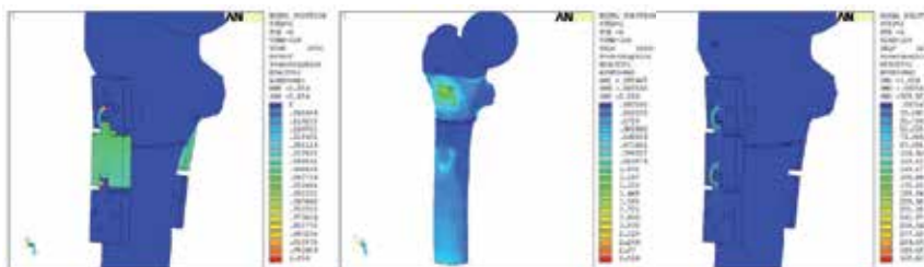
Fig. 21. Total displacements in the bone-implant assembly (a), von Mises stress in femur (b), von Mises in the element (c)
