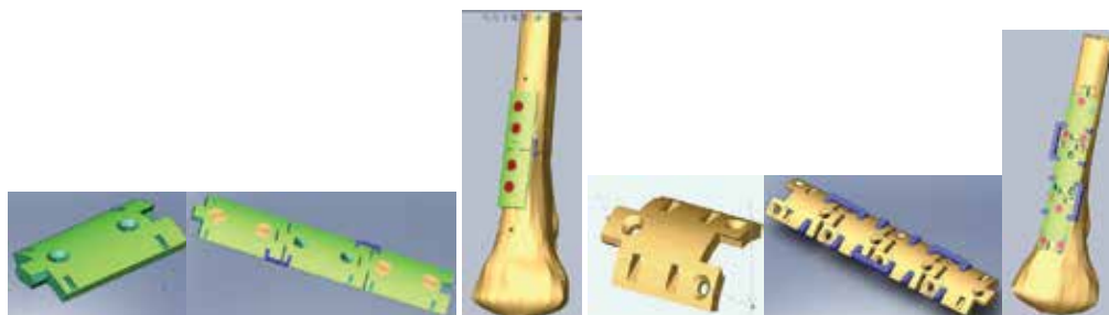
Fig. 16. Modules, plates and tibia-modular plate assembly for diaphyseal fractures
