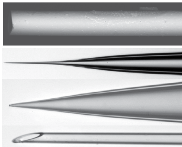
Fig. 2. Electron and optical microscopy images of pre-processed (top) and conventionally processed capillaries.
