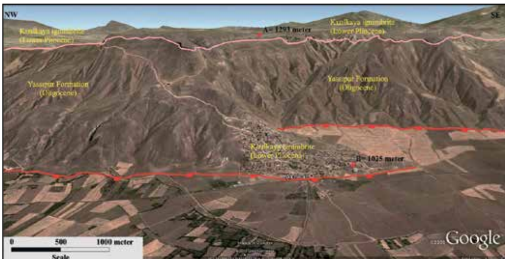
Figure 15. Google earth image of Kızılıkaya Ignimbrites displaced by Tuz Gölü Fault, in the vicinity of Akhisar Village; the amount of vertical displacement between the points A and B is 268 meters.
