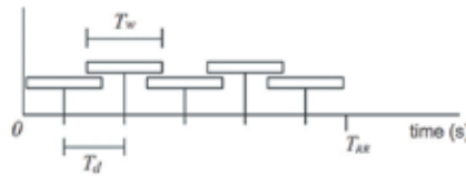
Fig. 5. Diagram illustrating the two aspects of temporal resolution. T_w is determined by the rotation time and reconstruction algorithm. T_d is determined by the heart rate and the number of reconstructed phases (five in this example).
