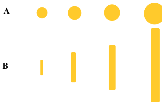
Figure 2. Schematic diagram of spherical (A) and rod (B) shaped gold nanoparticles.
