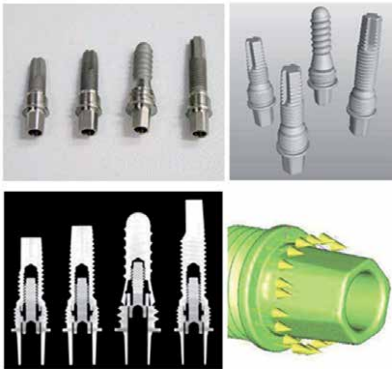
Figure 21. Four dental implants (top left), rendered point cloud (top right), cross-section of point cloud (bottom left) and detail to STL file imported to metrology software Calypso.
