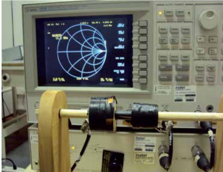
Figure 16. Free space measurement test set up.
