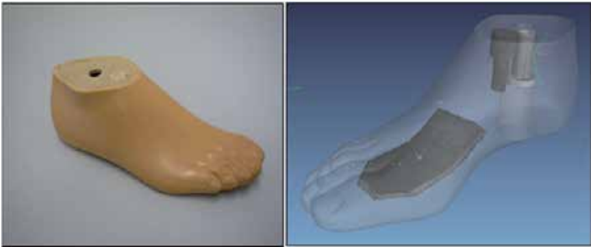
Figure 9. Epithetic foot and obtained 3D model (visible transparency of lower density material – soft surface plastic and wood).
