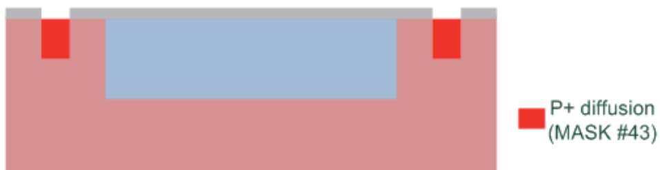
Figure 14. Guard ring get with P+ diffusion.
