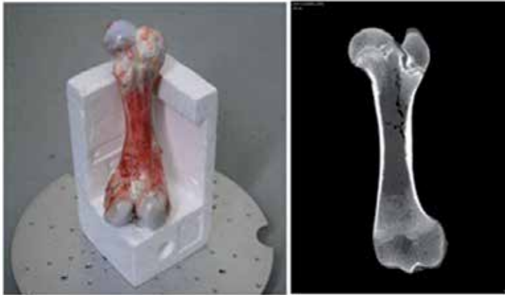
Figure 18. Pork femur (left) and its virtual cross-section (right).
