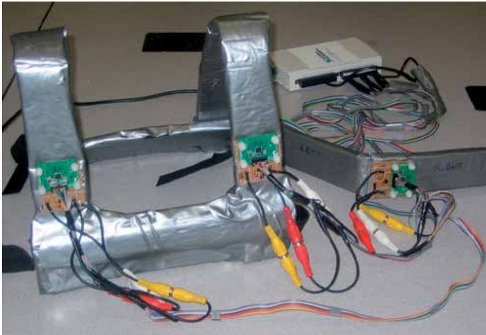
Figure 9. Instrumented harness providing input to the VR training system. Accelerometers attached to the shoulder harness are positioned on the trainee's shoulder blades, and the belt contains a third accelerometer, which is positioned on the lumbar region of the low back. [29]
