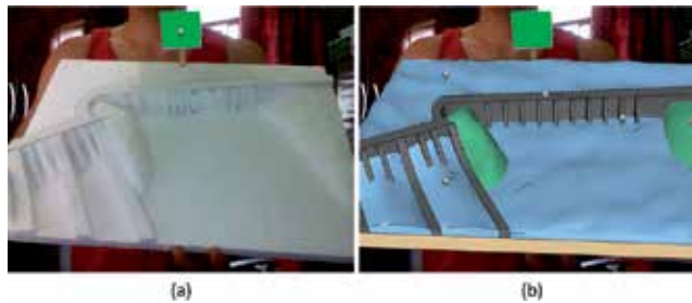
Figure 14. AR Spatial Tutor - Multimedia. (a) Mockup without AR layer and (b) with AR layer.
