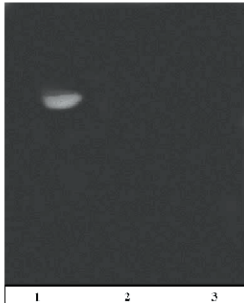
Fig. 4. Activity staining of SOD after conducting non denaturing PAGE. Staining was carried out according to the procedure described under Materials and methods Normal peroxisomes (Lane 1), peroxisomes post 90 days infection (Lane 2), peroxisomes post SAG treatment (Lane 3)
