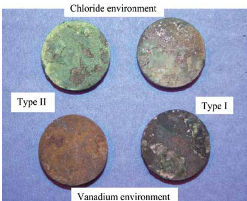
Fig. 5. As hot corroded superalloy IN 738 LC in marine and vanadium containing environments under type I and type II conditions
