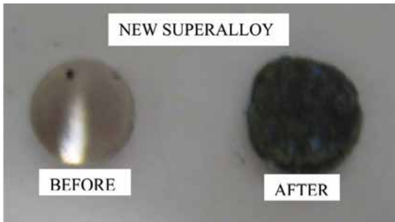
Fig. 8. Before and after hot corrosion in marine environment under type I conditions
