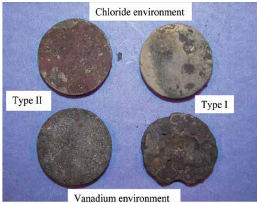
Fig. 4. As hot corroded superalloy SU-718 in marine and vanadium containing environments under type I and type II conditions
